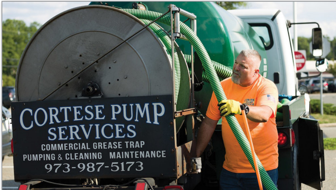
An electric reel with 300 feet of suction hose helps Cortese Pump Service technician Mike Toscana when he has to make a long run to a grease trap. It's much easier than running sections of hose.
